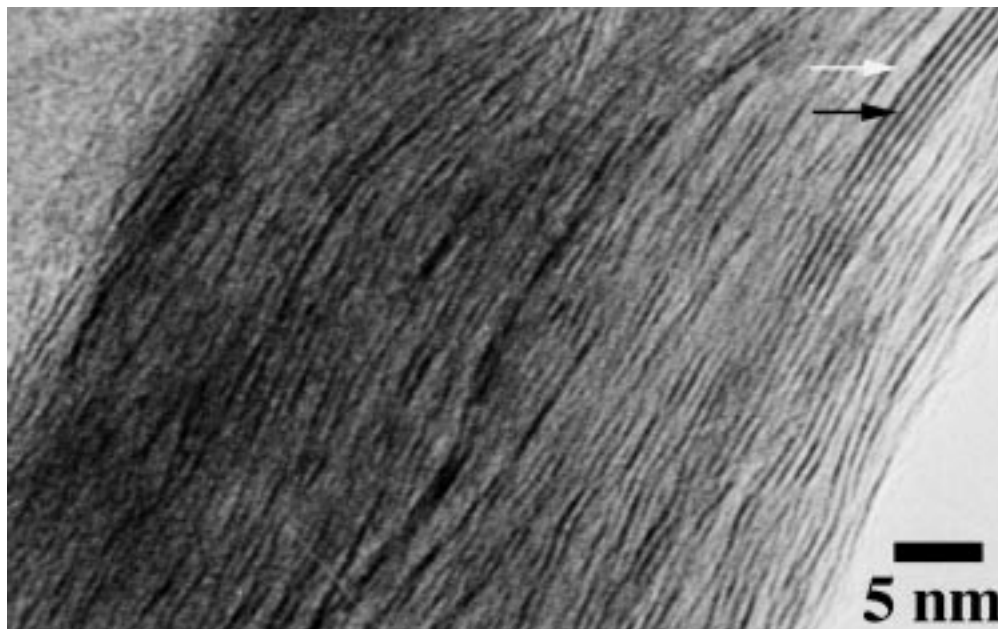
Figure 12. Significant degree of pillaring remains in the [\text{Co}_6\text{S}_8(\text{PPh}_3)_n]_{0.02}\text{MoS}_2 material after use as an HDS catalyst. The lattice constant for the pillared \text{MoS}_2 materials remains constant within experimental error before and after catalysis.
